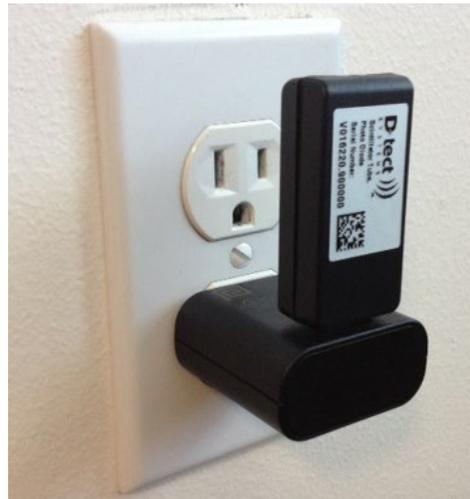
**Figure 11: DX-Link as a Repeater**
