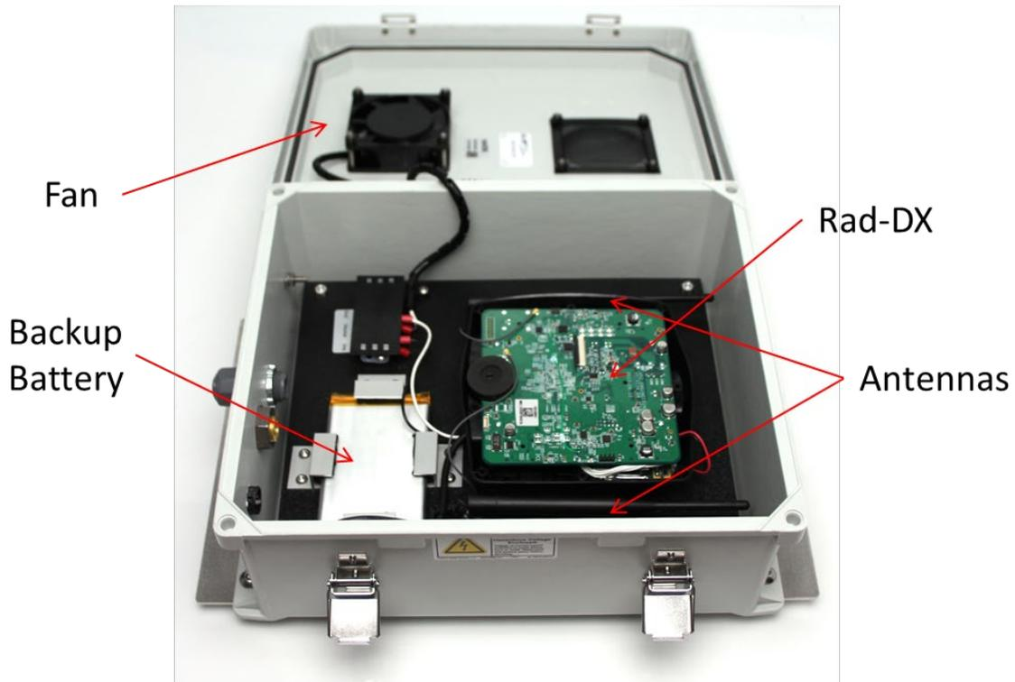
**Figure 5: Inside the NEMA Enclosure**
