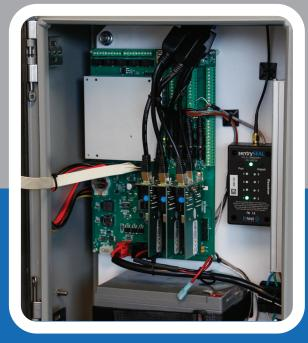
The principle of the Sentry-Seal is simple: a fiber-optic line is wrapped around the panel or door to be protected, if the fiber-optic line is broken, it activates an alarm. The Sentry-Seal incorporates proprietary encryption algorithms and tamper protection so that the device's transmissions cannot be spoofed, tricked, or disabled.
