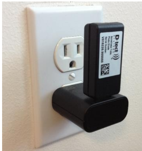
Figure 11: DX-Link as a Repeater
