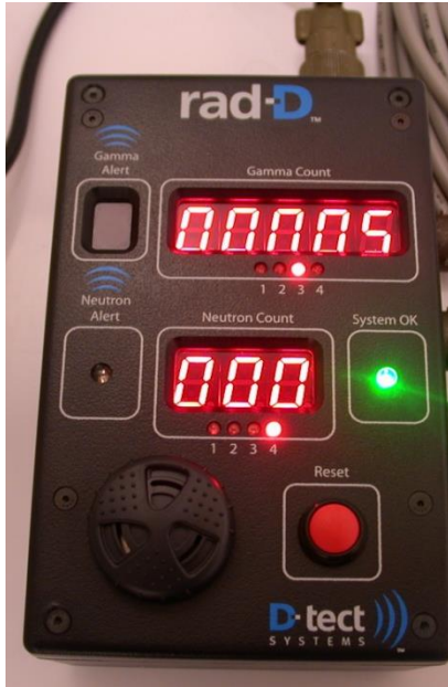
Figure 3. System 'OK' LED flashing green and gamma/neutron counts
