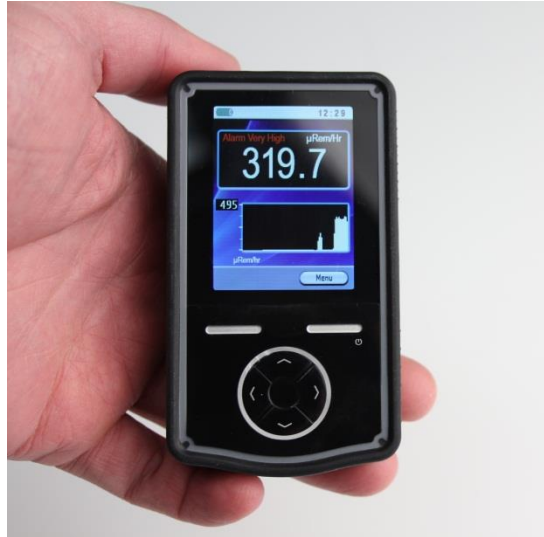
Figure 1: MiniRad-DX Handheld Radiation Detector
