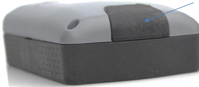
Figure 18: USB port location under protective cover
