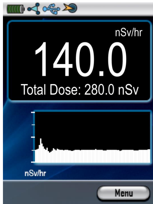
Figure 2: LCD Front Screen: Dose Rate and Graph
