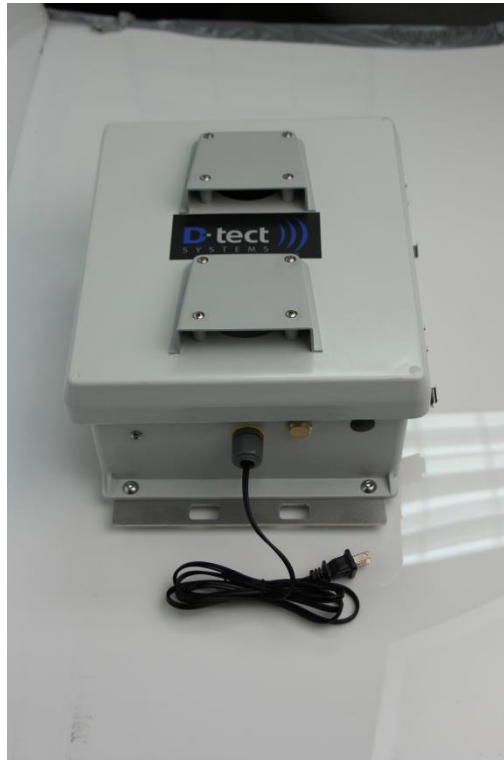
Figure 2 – Rad-DX NEMA Enclosure with Temporary Power Cable
