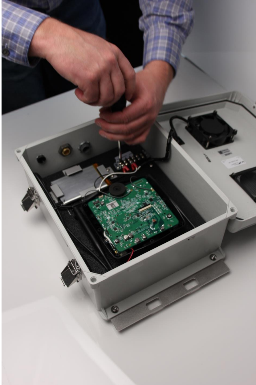
Figure 6 - Remove Power Cable
