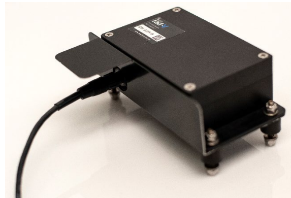
Figure 4: External Detector with Protective Shield
