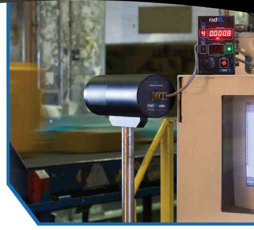
The Rad-D is a fixed-position radiation detector that is used to monitor doorways, driveways, and loading docks. It can inspect packages or luggage on conveyor belts and can be integrated with an X-ray machine or metal detector to increase detection capabilities.
