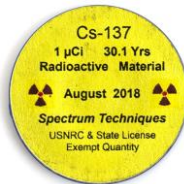
Figure 4.6. Cs-137 Check Source Labeled Side.
