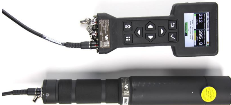
Figure 4.55. Cs-137 Check Source Position on Sensitive Gamma Probe.
