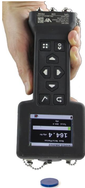
Figure 3.24. Base Unit Being Held Perpendicular to Suspected Surface.
