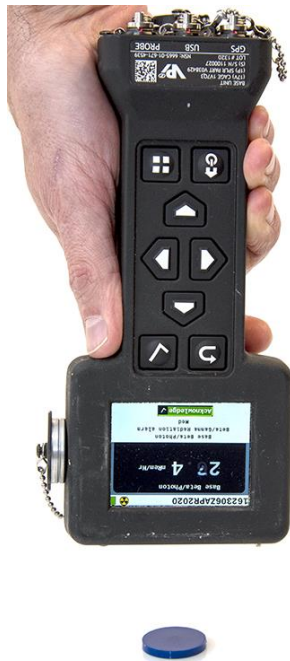
Figure 3.25. Beta Window Cap Removed and Placed on Side of Base Unit.
