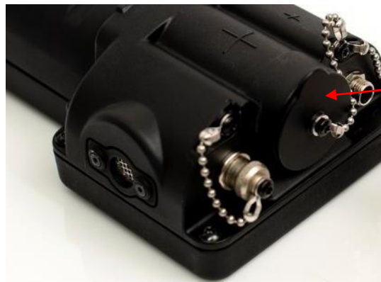
Figure 3.18. Beta Window Cap Installed.
