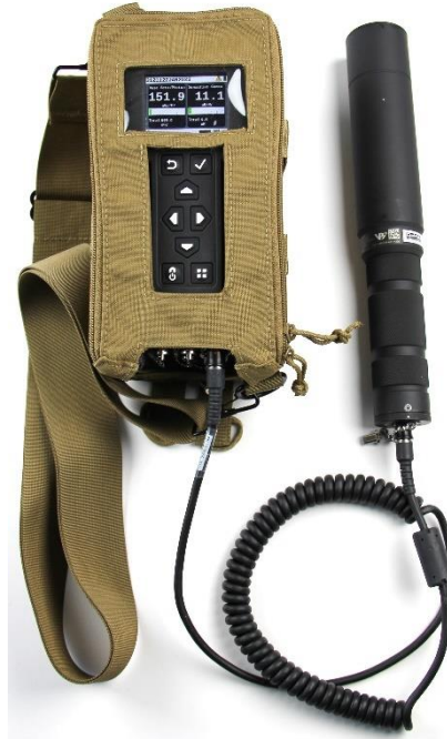
Figure 2.8. Base Unit Attached to Beta Photon Probe via Common Probe Cable.
