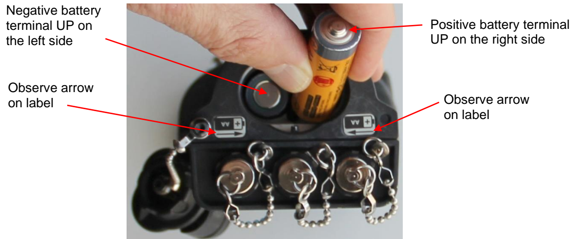
Figure 10.25. Battery Orientation.
