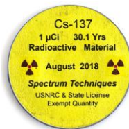
Figure 4.54. Cs-137 Check Source, Labeled Side.
