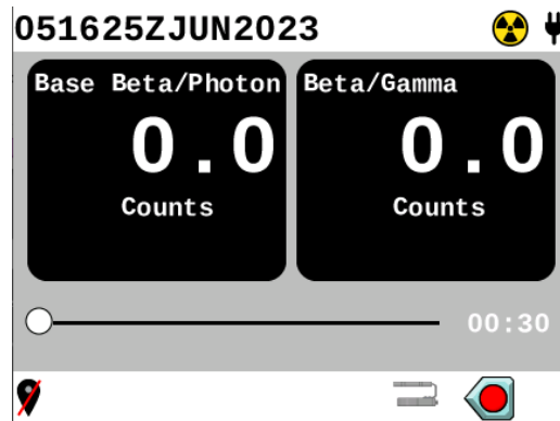
Figure 4.43. Home Screen Showing Base Unit and SABG Probe Reading Panels and Scaler Timer.
