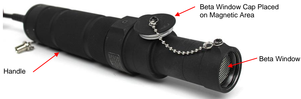
Figure 4.12. Beta Photon Probe with Beta Window Placed on Magnetic Area.
