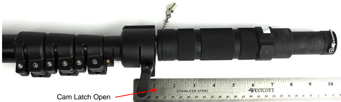
Figure 6.2. Cam Latch Open, Ready to Insert Probe into Probe Cup.
