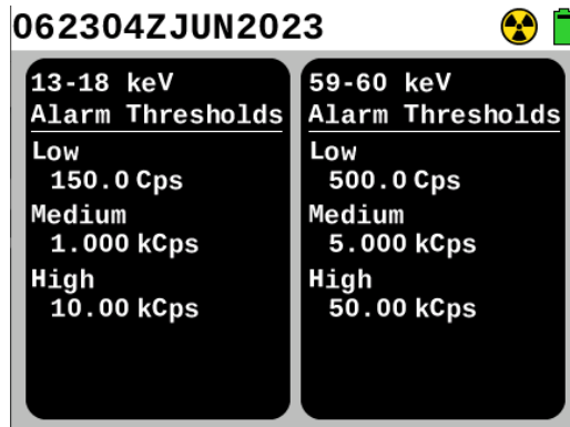
Figure 4.61. Example of Alarm Threshold Screen.
