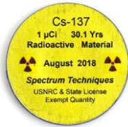
Figure 4.19. Cs-137 Check Source, Labeled Side.
