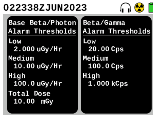
Figure 4.36. Alarm Threshold Screen Example.
