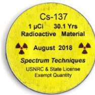
Figure 4.37. Cs-137 Check Source, Labeled Side.
