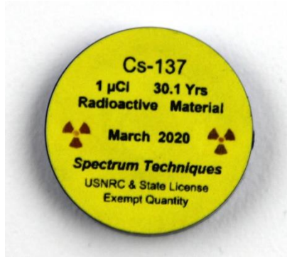
Figure 3.19. Cs-137 Check Source, Labeled Side.
