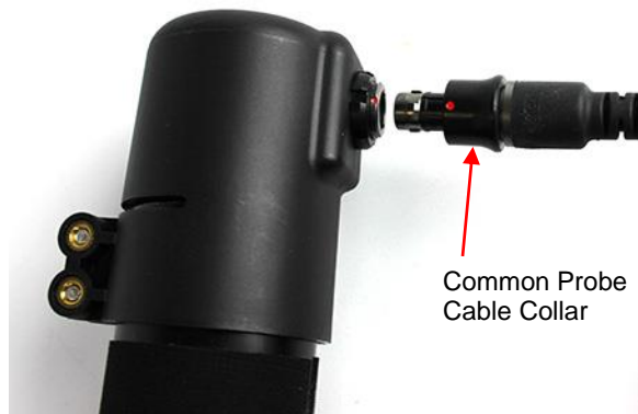
Figure 6.5. Connect Common Probe Cable to Telescoping Pole.
