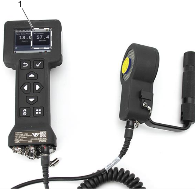
Figure 4.45. Scaler Mode Radiation Reading after 30 Seconds.
