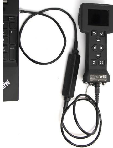
Figure 2.9. Base Unit Attached to Computer via Rad Extender Cable.
