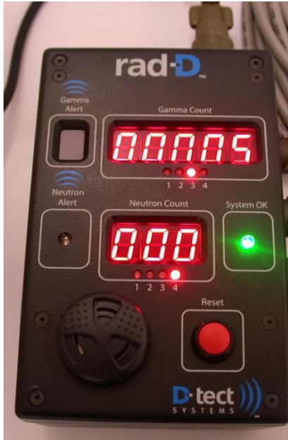
Figure 3. System 'OK' LED flashing green and gamma/neutron counts
