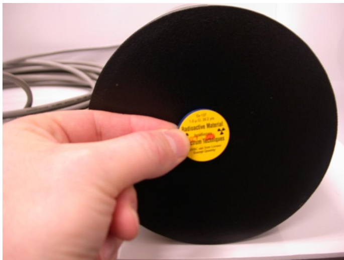
Figure 4. Radioactive source at the Detector and detecting level/counts.
