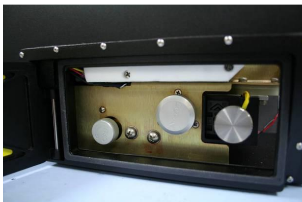
1. The Preconcentrator is the front knob in the side panel with wires.
