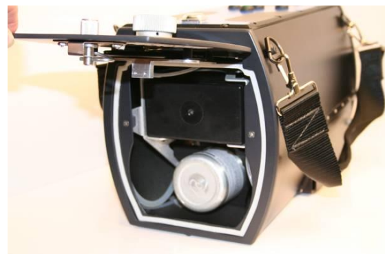
6. That's it. The helium tank is now installed.
