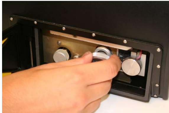
7. Screw the lid back. The reference chemical is now in place for testing.
