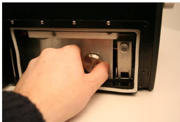
4. Take off the lid by twisting counterclockwise.
