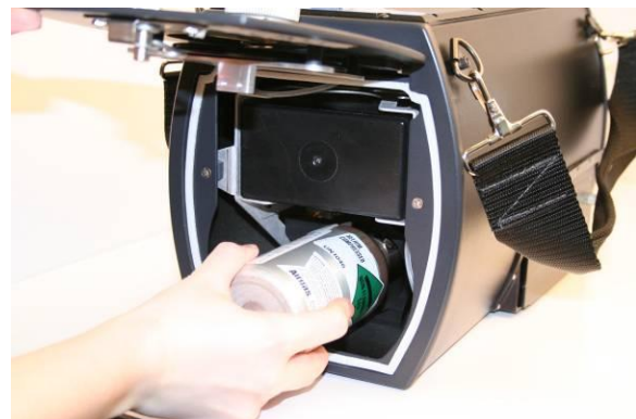
4. Slide the helium tank into the slot as shown until it touches the connector in the front.
