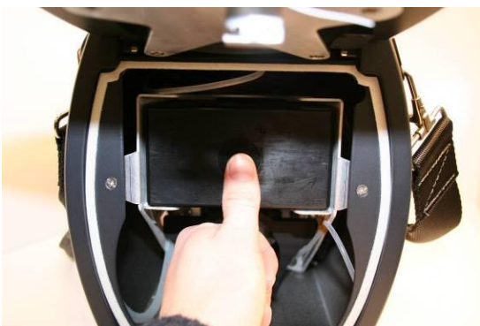
5. Push the battery in with your thumb. Apply a little pressure to make sure the battery seats.
