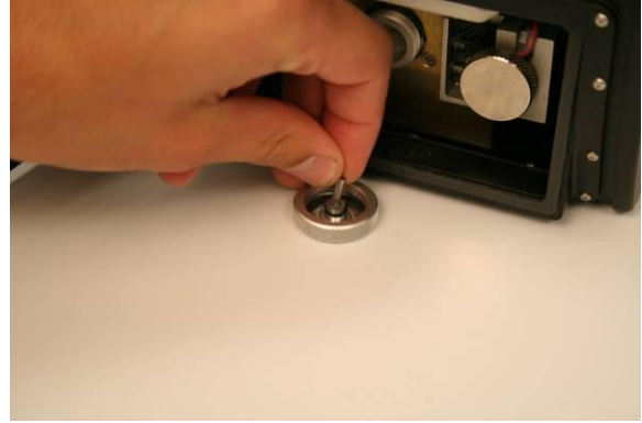
6. Pull out the old pellet and insert a new pellet with hole facing up.
