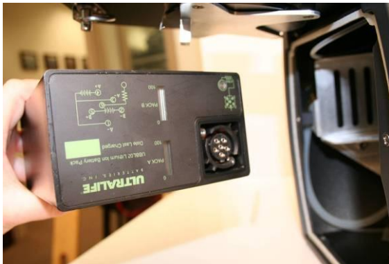
3. Hold the charged battery with the connector on the bottom and label on top.
