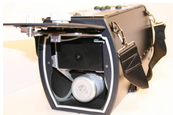
6. The charged battery is in place. Close and secure the door.
