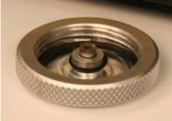
5. The reference chemical is contained in the little pellet in the lid.
