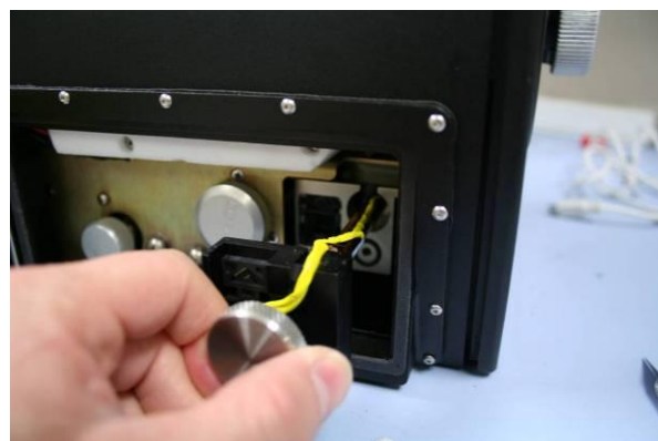
2. To remove, just twist the knob until the assembly can be pulled out.
