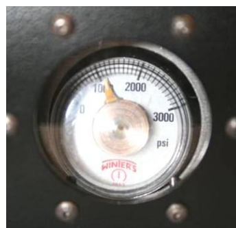
Step 2: Check the helium gauge for a reading of at least 300 PSI.
